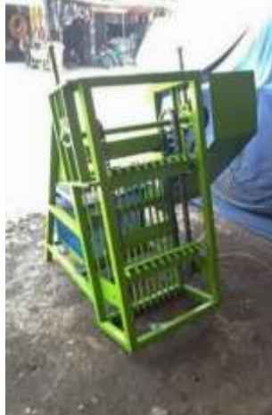
Figure 2. The results of making an automatic trash rake tool in the river using chain conveyor.
