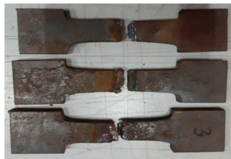
(a) Neutral variation specimen samples before the tensile test and (b) Neutral variation specimen samples after the tensile test.
