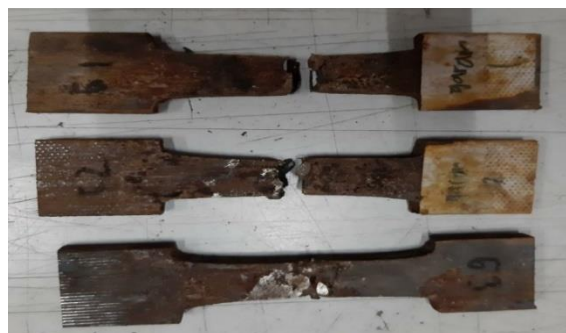
(a) Samples of variation of Brine before tensile test and (b) Samples of variation of Brine after tensile test.
