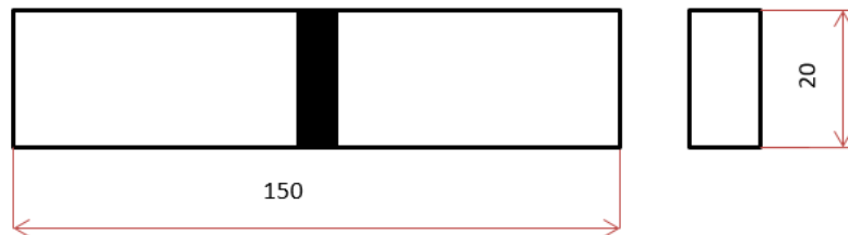
Figure 5. Bending Test Specimens (ASTM E23-02)
