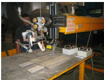
Figure 5. SAW Welding Machine
