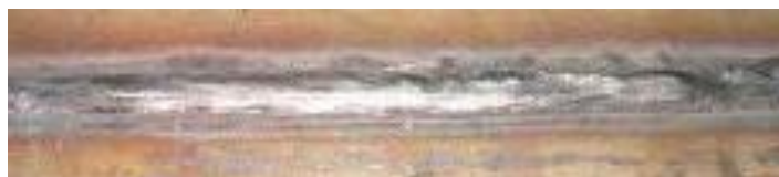
Figure 8 Welding Results with Ampere 410 A Volt 30
