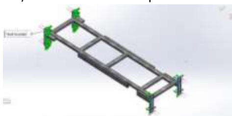
Figure 4.9 Selection of the type of support in the simulation
