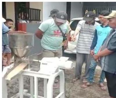
Gambar 1. Mesin Screw Extruder Kapasitas 25 kg
